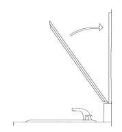
Clean the mirror with a 50-50 mixture of alcohol and water. Remove the backing from the tape. Be careful not to touch the tape to the mirror yet. Align Easy Frame® and gently press onto the mirror.
