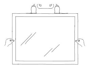
DO NOT APPLY FINAL PRESSURE to the frame yet. Inspect the alignment and if it is correct, apply direct pressure to Easy Frame®.
