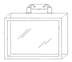
After applying the speciality tape, test fit Easy Frame® to the mirror. Check for obstacles that will affect installation. As a safety measure, if the stability of the mirror is in question, place several offset metal mirror clips on the mirror into studs.
