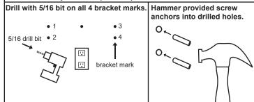
**STEP 7:** Affix brackets to wall. Ensure bent side of bracket is facing up and that pilot holes are level with bracket hanging height mark.
