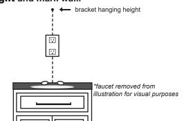
**STEP 3:** Measure between center point of bracket slots. This will be the spacing you use for brackets.
