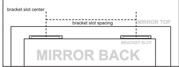
STEP 4: Level and center bracket slot spacing on your bracket hanging height orientation mark and make 2 marks for your bracket pilot holes.
