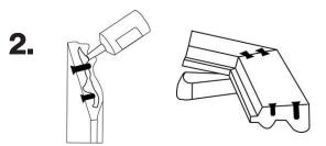
Choose a corner and apply glue to both pieces. With both glued pieces face down, level and align the corner and the routes. Depending on the profile, a door stop may be needed to level the frame.
