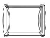
If necessary, a plastic shrink wrap can be used to pull all miters tight until the glue dries. Any excess glue that squeezes out on to the front of the frame can easily be picked off once the glue has fully dried.
